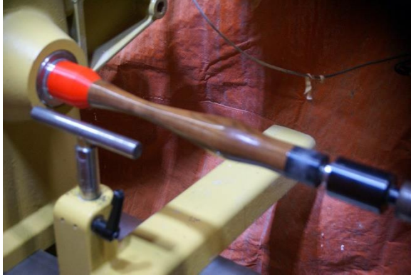
Picture #5 Adjusting the top of Spindle
